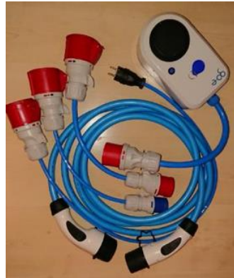
Figure 7: The Swiss Knife of the electro mobility: a mobile charger with cables and adaptors Source B.A.U.M. Consult
