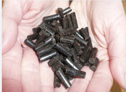
Pellets produced from sewage sludge, greenery waste and bark material within ENERCOM project
